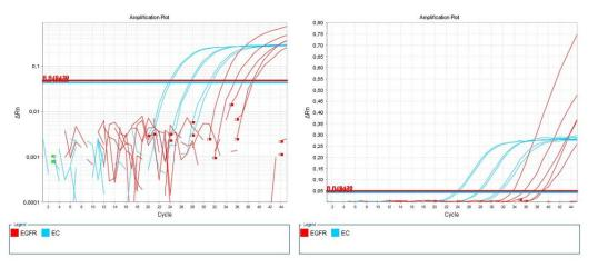
The automatic threshold is set correctly in the exponential phase of the amplification curves.
