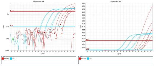
The automatic threshold of the Control (blue line) is set too low. The threshold of EGFR (red line) is set too high.
